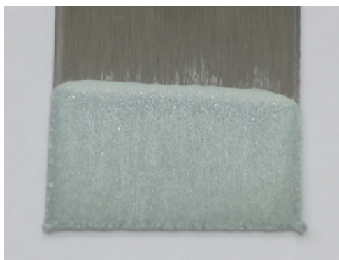
Fig. 6. Appearance of electrodeposited zinc (at 70 \text{ mA cm}^{-2} during 30 min) from the EPT stripping acid solution.
